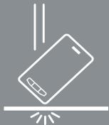
Hard drive disk failures and broken displays are common if a handheld, laptop or tablet is dropped. Rugged devices are designed to absorb and resist impacts from up to 3m.
